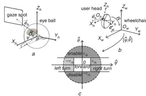
Fig. 3 Eye-gaze angles, head-to-wheelchair transformation, and wheelchair control scheme
