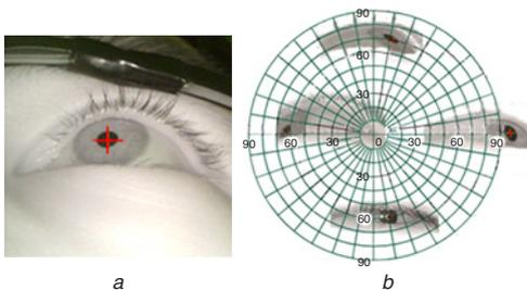
Fig. 2 Pupil's centre detected by EGT, and examples of eye-gaze angles from EGT
