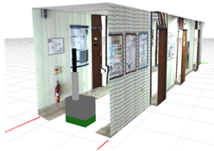
Fig. 6. Several views of real-time 3D visualized map while the robot explores in corridor of KAIST computer science building.
