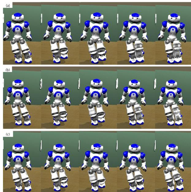
Fig. 3. Simulation snapshots of three kicking motions with different ball target positions.
