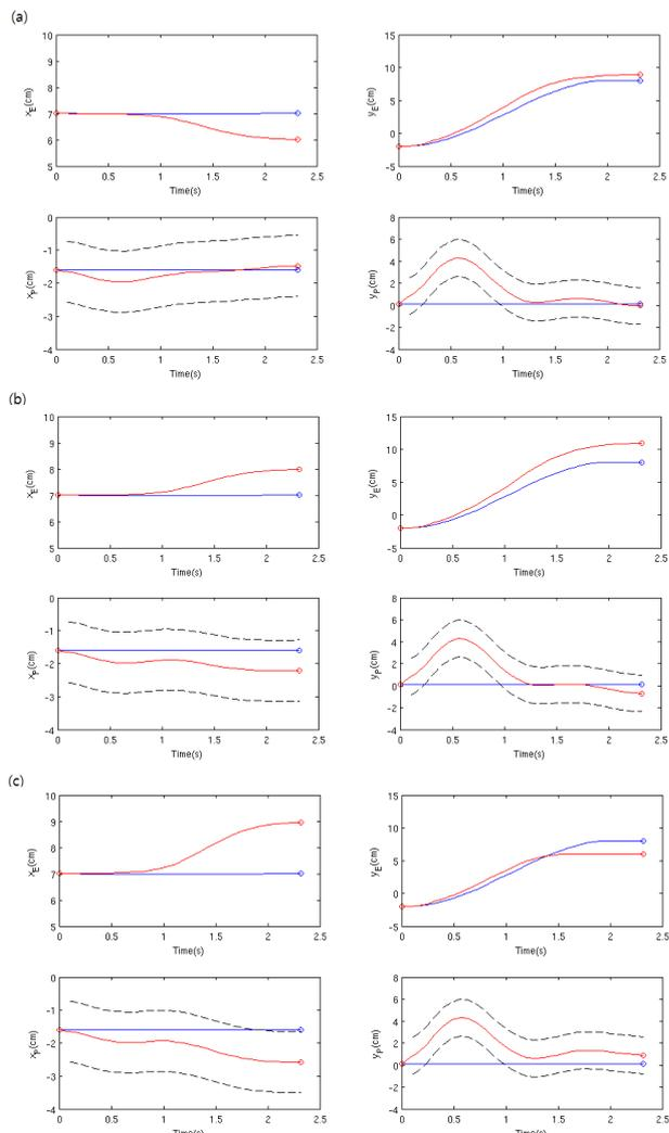
Fig. 2. Generation of three kicking movements ((a),(b),(c)). The blue line indicates a principal kicking movement from demonstration, and the red line represents a new kicking movement to reach a new ball position. Each subplot shows the trajectories of  $x_E, y_E, x_P$  and  $y_P$ . Dotted lines indicate the upper and lower bounds (as in (8)).
