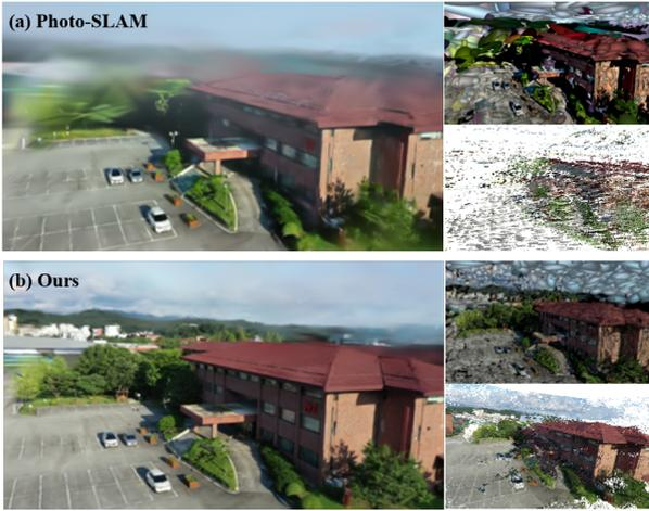
**FIGURE 1.** Rendering results of (a) Photo-SLAM [21] and (b) our method. The optimized Gaussian points and the estimated point cloud for each method are shown in the upper right and lower right, respectively.
