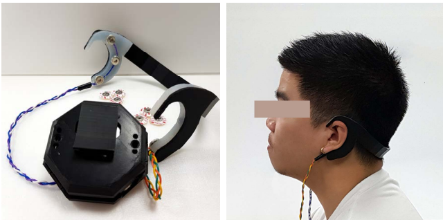
Figure 2. (left) The Ear-EEG acquisition device. (right) A subject wearing the device.
