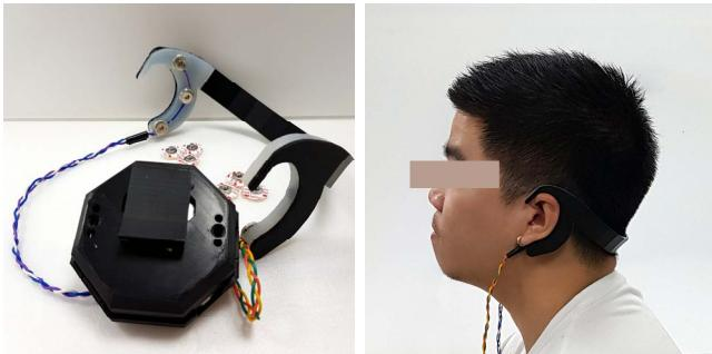
Figure 2. (left) The Ear-EEG acquisition device.
