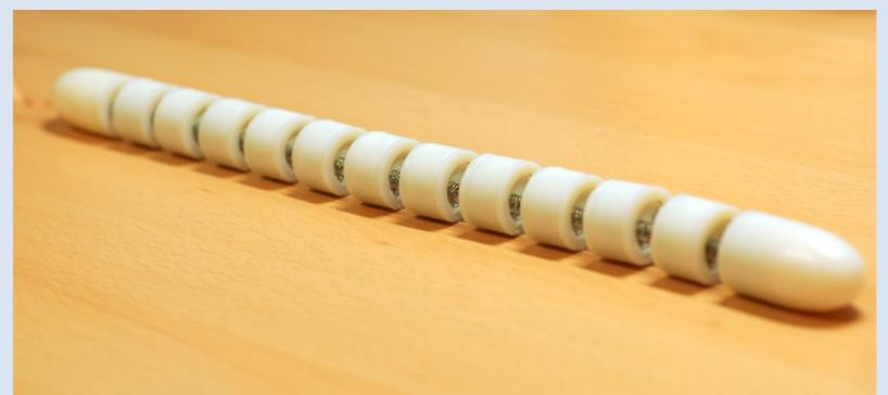
Figure 4. Implemented robot hardware prototype. (Length: 30 cm, Weight: 100 g)
