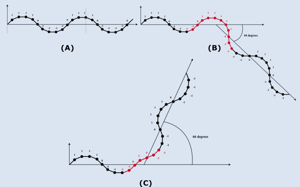
Figure 3. Sequential code for (A) Forward motion (1 1 0 -1 -1 -1 -1 0 1 1), (B) S1 right turn (1 1 1 1 0 -1 -1 -1 -1 0 1 1), and (C) S2 left turn (1 1 0 -1 -1 -1 -1 0 1 0 -1 -1 -1 -1 0 1 1).
