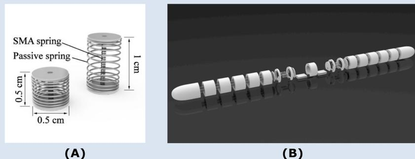
Figure 2. Proposed design of (A) linear actuator based on thermal SMA, and (B) whole robot assembly.
