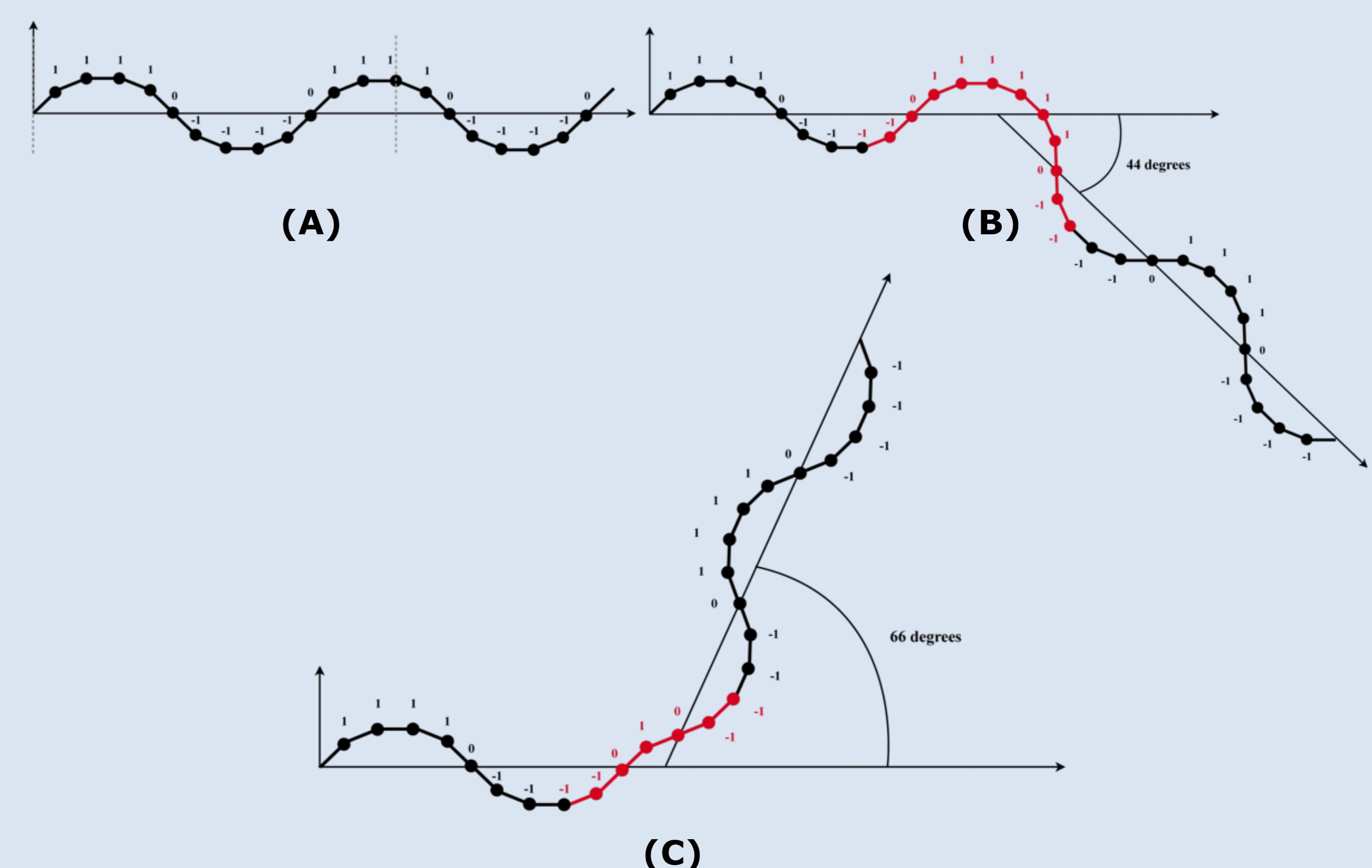
Figure 3. Sequential code for (A) Forward motion (1 1 0 -1 -1 -1 -1 0 1 1), (B) S1 right turn (1 1 1 0 -1 -1 -1 -1 0 1 1), and (C) S2 left turn (1 1 0 -1 -1 -1 0 1 0 -1 -1 0 1 1).
