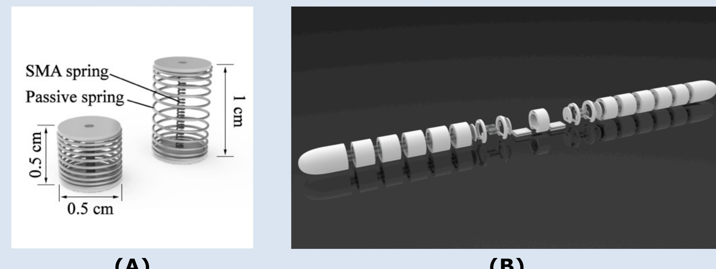
Figure 2. Proposed design of (A) linear actuator based on thermal SMA, and (B) whole robot assembly.
