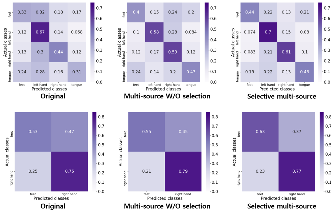
Fig. 7. A confusion matrix indicating grand average accuracy results for having each subject evaluated as a target domain. The results of when no source subject was used for domain adaptation, using all subjects for loss measure of our domain adaptation, and using the optimal number of source subjects on each epoch for loss measure are presented. The upper plots represent the results from the BCICIV dataset, and the lower plots represent the results from the ARA dataset.
