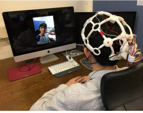
Fig. 3. Subject wearing custom-made 3-D-printed headgear with OpenBCI 32-bit board kit while performing the experiment.
