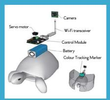
The entire human-turtle setup is as follows: A head-mounted display (HMD) is combined with a BCI to immerse the human user in the turtle's environment. The human operator wears the BCI-HMD system, while the turtle has a 'cyborg system'—consisting of a camera, a Wi-Fi transceiver, a computer control module and a battery—all mounted on the turtle's upper shell. Also included on the turtle's shell is a
